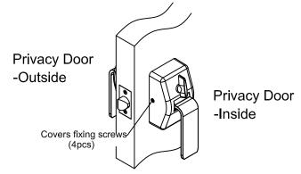
6. Fastened both covers with screws as indicated on either sides of covers, total 4pcs and check the Privacy Indicator is correctly functions.
