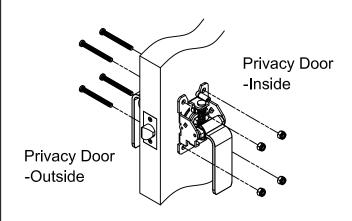
4. Make sure both inner and outer push/pull chassis's are flush to door panel, and inserts all four 1/4"-20x2-15/32" screws onto 4 bolt through holes from outer chassis and fastened with 4pcs 1/4"-20 hex hex nuts on inner chassis.
